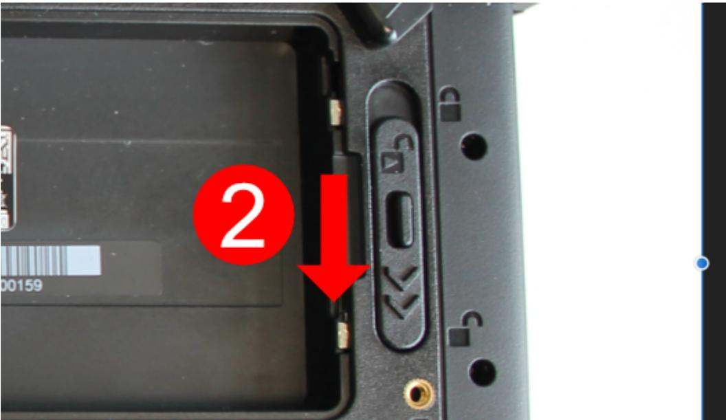
3. Now insert the battery as indicated. Make sure that the contacts of the battery are on the correct side of the device.
