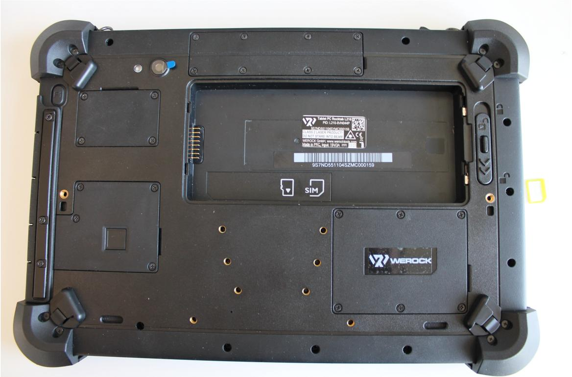
2. Slide the Micro SIM card into the SIM card slot with the contacts facing the device and the bent side facing forward until it clicks into place
