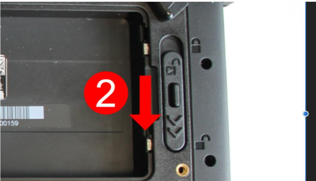
3. Now remove the battery as indicated and insert the new battery in the same way.
