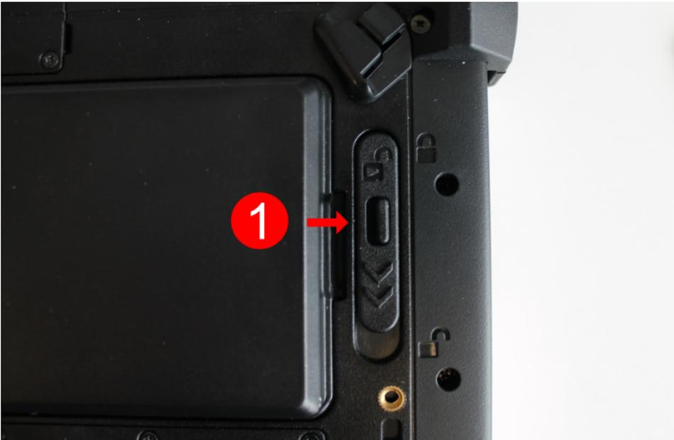
2. Make sure that the locking mechanism (number 1 in the operating and display elements diagram) is set to unlocked. You can tell this because the slider is closer to the "open lock" symbol than "locked lock".
