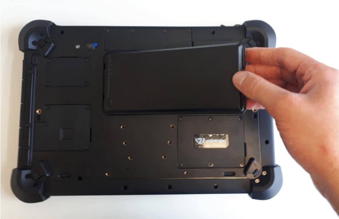
4. Finally, lock the locking mechanism and close the safety catch.
