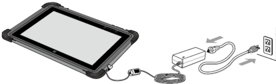
When the power adapter is plugged in, the battery begins charging. The battery LED indicator on the tablet computer shows various states. Please refer to the description of the LED indicator.
