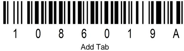
**Add Tab:** If this option is activated, the barcode scanner adds a tab after scanning a barcode. This corresponds to pressing the "Tab" key on a keyboard. The scanned data is left in a single line, with a tab inserted between the individual scanned data.
